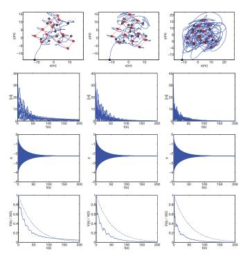
Fig. 3. Simulation results for different values of K with h=0.9: left-column (K=0.05), middle-column (K=0.15) and right-column (K=0.85). First row: trajectories followed by each agent. Second row: Velocity norms of each agent  $||v_i||$ . Third row: Estimation of the angle  $\hat{\phi}_i$ , and Fourth row: Normalized cost function (solid-line) vs decay rate (dashed-line)
