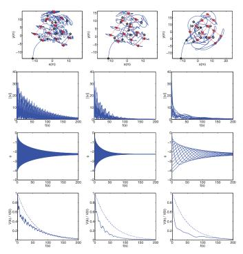
Fig. 4. Simulation results for different values of h with K=0.15: left-column (h=0.75), middle-column (h=0.9) and right-column (h=0.98). First row: trajectories followed by each agent. Second row: Velocity norms of each agent  $||v_i||$ . Third row: Estimation of the angle  $\hat{\phi_i}$ , and Fourth row: Normalized cost function (solid-line) vs decay rate (dashed-line)
